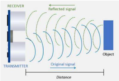
Figure 13 - Operation principle of distance sensor
