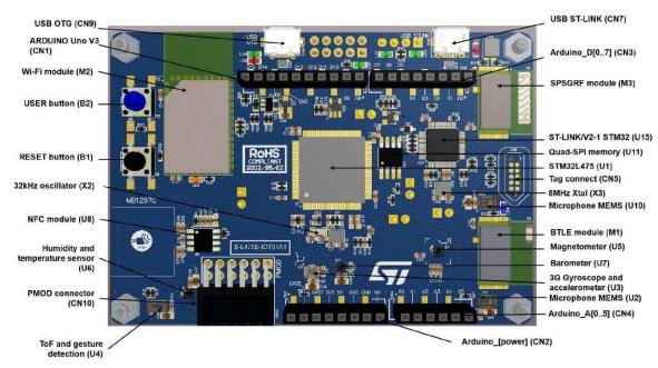
Figure 14 - Schematic layout of the IoT board. At top-left side can be seen the USER button (B2)
