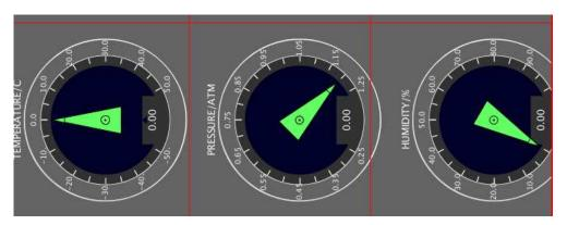
Figure 15 - Dashboard of a basic weather station monitoring temperature, atmospheric pressure and relative humidity
