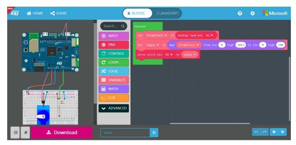
Figure 12 - Example program in MakeCode on how to control servo and LEDs
