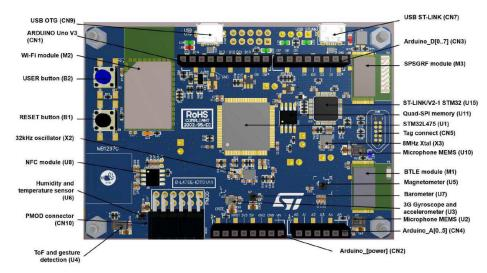
Figure 17 - Schematic layout of the IoT board
